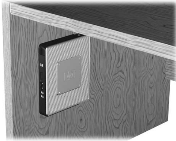
Figure C-8 Thin client mounted under desk
