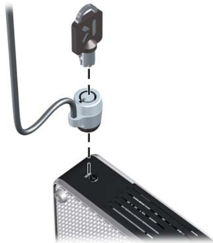
Figure B-1 Securing the thin client
