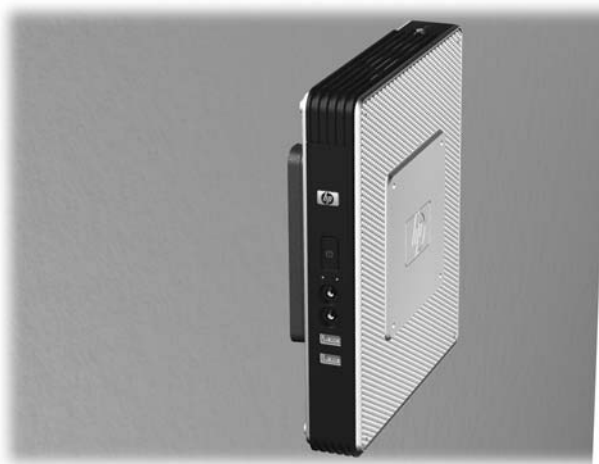
Figure C-7 Thin client mounted on wall
